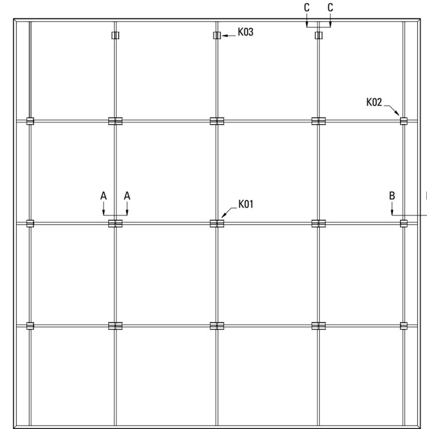
SOLUZIONE CON MONTANTE PER ALTEZZE FINO A 10 M / SOLUTION WITH POST FOR HEIGHTS UP TO 10 M
