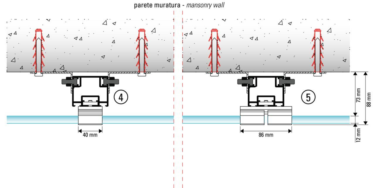
**SEZIONE ORIZZONTALE . SOLUZIONE CON COIBENTAZIONE SULLA PARETE / HORIZONTAL SECTION, SOLUTION WITH INSULATION ON WALL**
