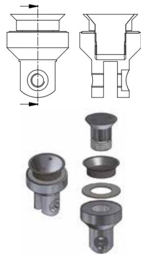
attacco svasato per PA: 01-02-03 / countersunk connection for PA: 01-02-03
